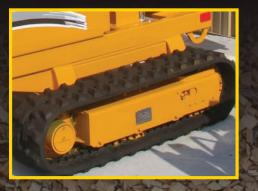
**Self-Propelled** Available with **rubber track undercarriage**, the Model 250XP can be taken right to the trees.
